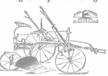
Made with the fewest parts-no frame. Strongest plow of its type made. Weight properly distributed—no drag on bottom.
