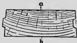
FIG. 1.—A section of a stave. The face a is \frac{1}{8} to \frac{1}{4} less than b .
