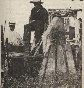
THIS ugly machine for pulling flax was invented by an Ontario preacher. It is here seen at work in a York county field, man-ridden, tractor-hauled, ugly—but expected in future to be efficient.
