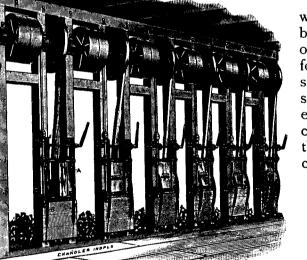
When two or more knives are run with one belt, all must stop when the belt is stopped to set bits or from any other cause. Our Machine has a belt for each knife, hence but one knife stops at a time. This great advantage should not be overlooked by purchasers. Time is money. Our Machine cuts more excelsior in a given time than any other machine. Get our circulars and prices.
