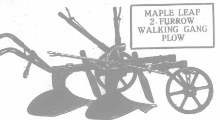
Y actual tests, in competition, this 2-furrow walking B gang plow plowed two furrows 9 inches wide and six inches deep with but 25% heavier draft than a single-furrow walking plow, in the same soil and with the same horses and plowman. And it was heavy soil at that. To YOU this means that three horses and one man, with this plow, will do as much as four horses and two men with two one-share walking plows-and the plowing will be
