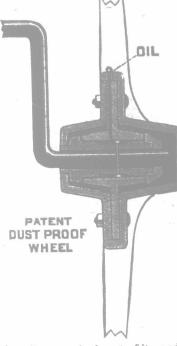
it; oil cannot leak out of it; and the axles cannot spring nor weaken a little bit. Once oiled these wheels run silently and perfectly for days-another lightdraft feature gained by reducing friction. Send for details of this practical device—it will pay you.
