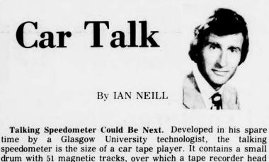
drum with 51 magnetic tracks, over which a tape recorder head moves laterally in accordance with the speed measurement, selecting the appropriate pre-recorded track. The "talking" meter can be set to give continuous speed announcements. It can also be activated by a small column mounted switch. Other controls could select voltage, temperature, oil pressure or other readings. The device, according to the inventor, could be mass produced for
