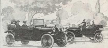
Long-Stroke "32" Touring Car, \$1,000. F.O.B. Windsor, including equipment of windshield, gas lamps and generator, oil lamps, tools and horn. Three speeds forward and reverse; centre control; sliding gears. Four cylinder motor  $3\frac{1}{2}$ -in, bore and  $5\frac{1}{2}$ -in, stroke. Bosch magneto. 106-in, wheelbase,  $32 \times 3\frac{1}{2}$ -in, tires. Color, Standard Hupmobile blue.
