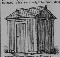
siding. The following materials wil build it: Fourteen pieces 2 by 4, 1+ feet; two pieces 2 by 6, 16 feet; two pieces 2 by 6, 12 feet; five pieces 2 by 4, 12 feet; 235 feet drop, siding, three bunches shingles, 60 feet six inch crown molding, 100 feet roof boards, four boards 1 by 12. 14 feet; two pieces six inch sewer pipe.
