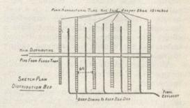
The size of the flush chamber is therefore directly governed by the size of the distribution bed, and the best results are obtained when the bed is flushed once or at the most twice, in the 24 hours.
