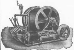
This is a view of our combined friction drum and brake and reversible link motion hoist. The most economical mining hoist built.
