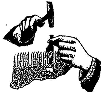
**Directions.**—Place the Set on the point of tooth as shown in the above cut, and strike a very light blow with a tack hammer. If you require more set, file the tooth with more bevel. If you follow directions you cannot make a mistake. Be sure and not strike too hard a blow, and it will set the hardest saw.
