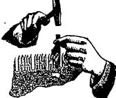
**Directions.**—Place the Set on the point of tooth as shown in the above cut, and strike a very light blow with a tack hammer. If you require more set, file the tooth with more bevel. If you follow directions you cannot make a mistake. Be sure and not strike too hard a blow, and it will set the hardest aw. 40 cents each.
