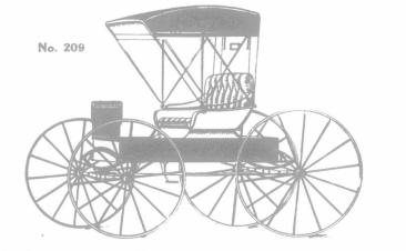
The body of this particular Buggy is made from choice Whitewood, with matured Ash frames, and steel corners if desired. It is handsomely trimmed with No. 1 leather, has full spring back and cushion. Top is made of finest 26 ounce rubber in 3,  $3\frac{1}{2}$  or 4 bows as desired.
