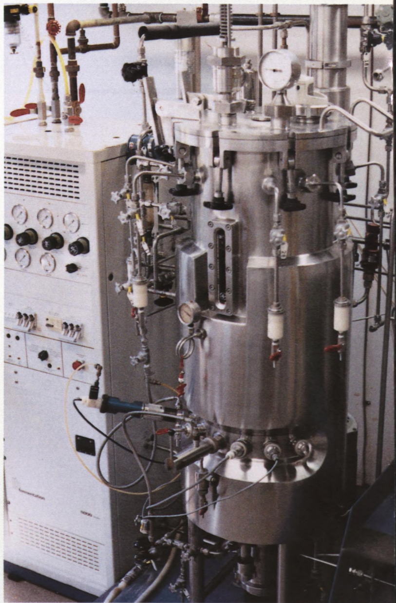
Production of vaccines using fermentation equipment. (Microtek Research and Development Ltd.)
