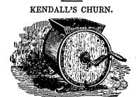
This is a churn much used in the States, and from its simple, compact, portable shape, we are inclined to think it is both cheaper and better than many of those new fangled contrivances with high sounding names, such as the "Thermometer Churn," "Atmospheric Churn," &c. &c. The The shaft passing cut needs no explanation. wings, which, by turning the handle, give motion to the cream.
