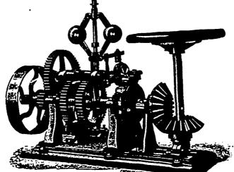
Any deviation from the correct speed, however slight, affects the action of the governor upon the gate, and it quickly brings the speed up or down to its proper point.
