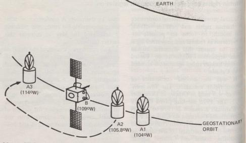
Move of Telesat's satellite Anik-A2 to collocate with Anik-A3.
