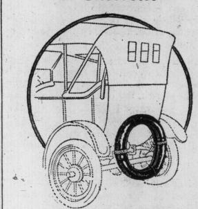
The Carrier is of black Japanned iron, has two arms, and bracket for lamp and license, and if necessary will carry two tires.
