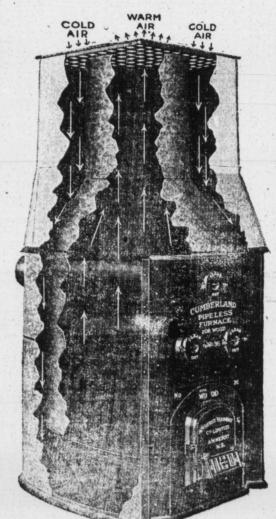
The Cumberland Pipeless Furnaces is ideal for most churches and halls because the moment the fire is started it immediately floods the building with warm direct heat. No time wasted heating pipes or water the Cumberland goes into action at
