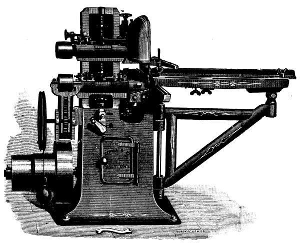
This is an entirely new style of Tenon Machine. The frame is cast in one piece, and the working parts stand solidly on a pedestal, avoiding
