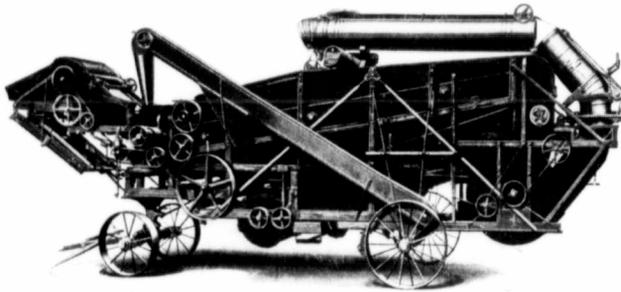
THE THRESHER with the big Cylinder of heavy Construction. Concave spikes placed so as to give least necessary clearance while allowing grain to pass between and effectually preventing heads going through with the grain. Shaft supported in Self-adjusting boxes. If level of machine is disturbed, the Cylinder is still bound to run true and even.
