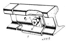
with a single circularly extending cam incline and a locking shoulder adapted to engage with the teeth of the washer.
