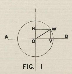
end of the stroke; neglecting the disturbance caused by the obliquity of the connecting rod, which is unnecessary to consider in any existing type of locomotive, these forces are identical with that caused by a corresponding mass at the crank pin, with the exception that they have no vertical effect.
