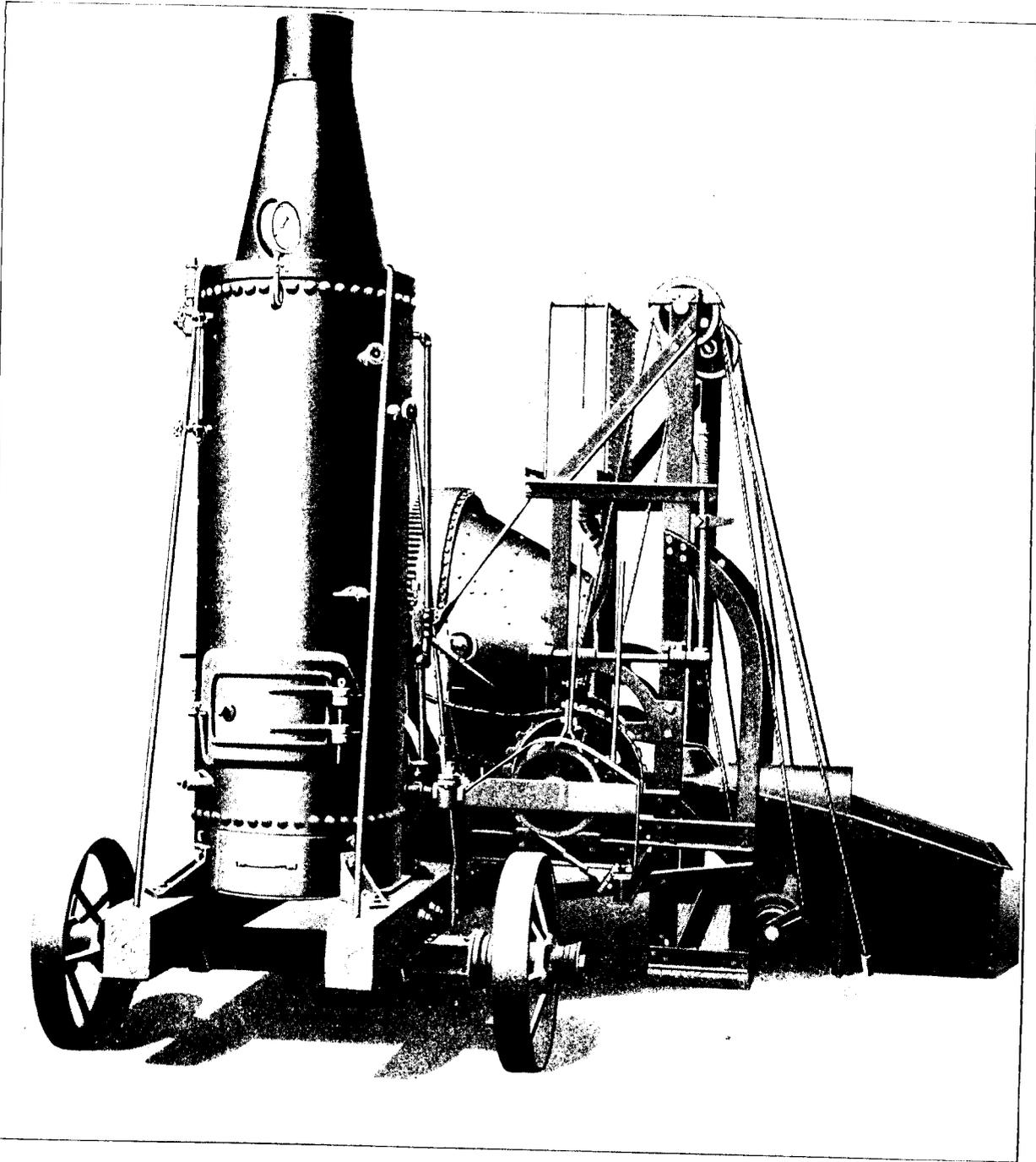
We illustrate one of our Portable Smith Mixers with our Patent Loading Device attached. This invention effects a great saving in time. It can also be used as an elevator to any desired height.
