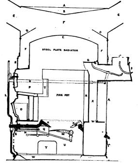
Marks a new era in the sanitary warming of our houses. The objections that have heretofore been urged against hot-air furnaces are entirely overcome in this apparatus. The vital point of superiority consists in covering the entire fire chamber and fines by an impervious drum of heavy steel plate, securely rivited. By this arrangement the escape or leakage of gases is an impossibility, while, by the system of flues used, the maximum quantity of heat is secured.
