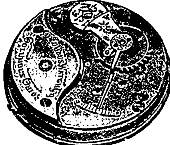
18 Size, Gilt.—No. 21, Hunting, or No. 91, Open Face, pendant set, 11 jewels, upper holes jewelled, tempered hair spring, sunk seconds dial.
