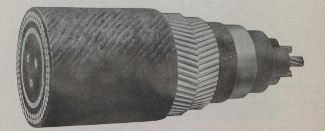
The longest paper insulated Sub-marine Power Cable on the Continent (supplied and installed by The Canadian British Insulated Co., Ltd., for the King Edward Park Company,) No. 6 B. & S. Gauge, 3 conductor, paper insulated, lead covered double wire armoured and juted.
