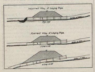
safe to raise it, while the lower end should be below the bed of the stream, say, 6 in. to 2 ft., depending upon the diameter of the pipe and surrounding circumstances, thus getting as great a fall in the pipe as is possible in each location. The
