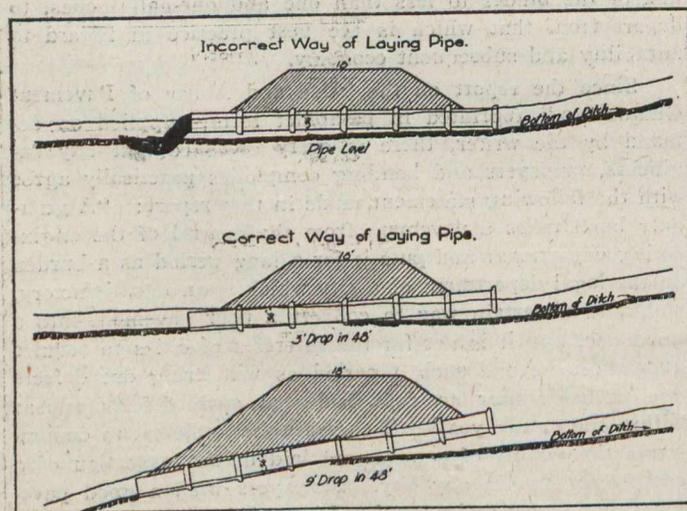
safe to raise it, while the lower end should be below the bed of the stream, say, 6 in. to 2 ft., depending upon the diameter of the pipe and surrounding circumstances, thus getting as great a fall in the pipe as is possible in each location. The
