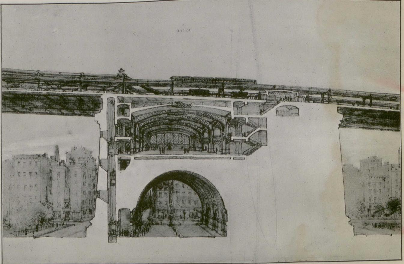
SECTION SHOWING STATION IN ANCHORAGE OF MANHATTAN BRIDGE, EAST RIVER, NEW YORK.
