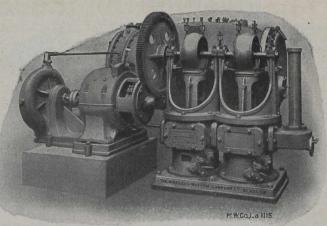
Surface Condenser with 2-throw Edwards Air Pump and Centrifugal Circulating Pump
