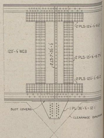
Fig. 4.—Detail of Web Splice and Web Hanger Plate.
