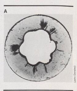
These cross sections of high-voltage power cables (A is across the cable, B is along it) show the developing "trees" in the insulation that eventually cause the cable to short-circuit.
