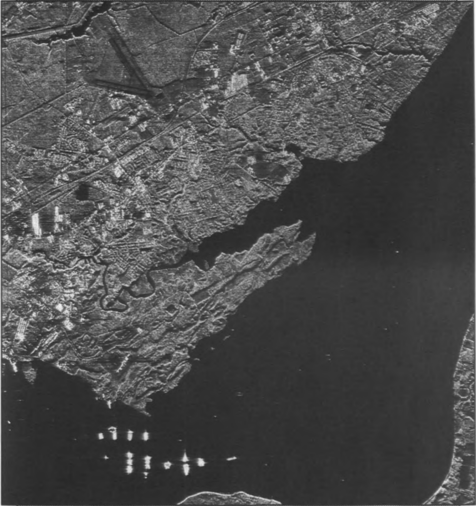
Figure 19 Synthetic Aperture Radar Imagery of Tethered Destroyers
