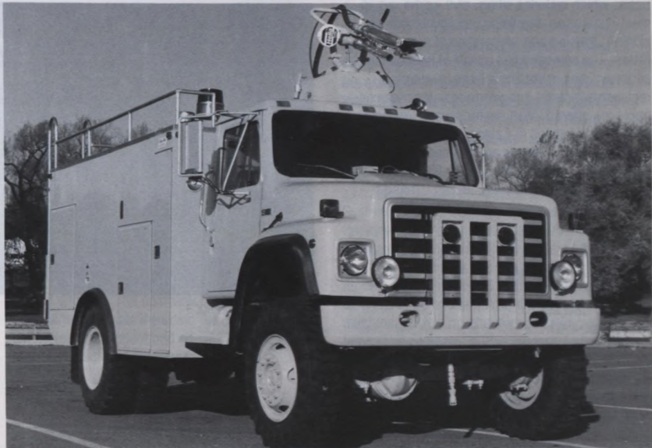
The "Foam Boss" 1200 L/135 kg dual agent rapid intervention vehicle
