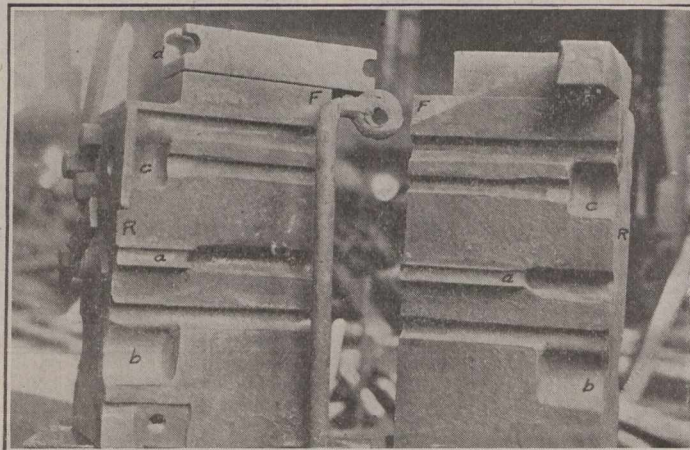
Fig. 2.—Dies for Forging Grab Iron in Forging Machine.
