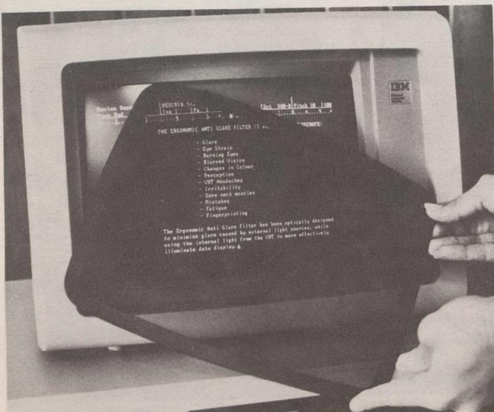
*The Ergonomic Anti-Glare Filter from Reach Industries has been optically designed to minimize glare from external light sources.*
