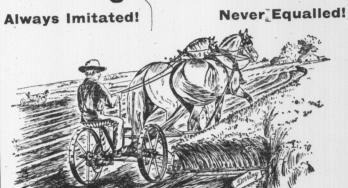
There is no waste of power or lost motion in the Deering Perfect Bearings, direct transmition of power and serrated ledger-plates make the action of the "positive that it will start cutting in any grass as soon as the tugs tighten on the k
