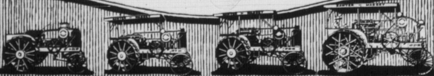
Four Cylinder Sawyer-Massey Gas-Oil Tractors *Kerosene Burning*
