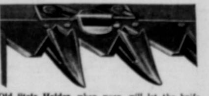
Old Style Holder, when worn, will let the knife rise up from guard plates, allowing grass to get in between and clog the knife
