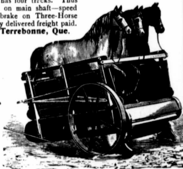
Three-Horse Tread Power with roller bearings.
