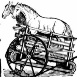
Two-Horse Tread Power with roller bearings
