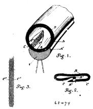
pneumatic tire having a pair of narrow primarily-flexible bands of diagonally-woven wire fabrics in its sides, the inflation of the tire causing a distortion and consequent rigidity of the bands, substantially as described.
