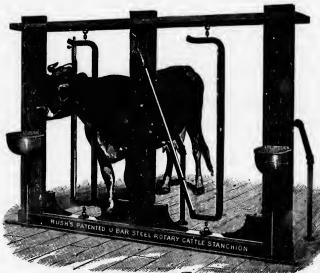
Above cut illustrates a good method of fastening Stanchion to cement work. A piece of iron 5-16 x 1 1-2 inch or heavier is formed into a Ushape about three inches wide and four inches deep with bolt passing through holes in both ends and placed in cement work as illustrated in cut.
