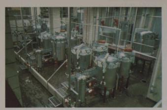
After the fermentation stops, the brew is filtered to remove the yeast.
