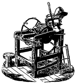
The drum is revolved by a lever operated by the left hand, and the nailer by another worked by the right. This nailer far surpasses anything of its kind in use. The nails are picked up, passed down a shute, and placed in position on the up stroke of the lever, and driven home on the return. By a rotary saw attachment, designed by Mr. MacMillan, the covers and bottoms are made with great rapidity.
