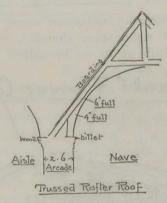
is to be flush with the wall, as it ought to be. The roof in the above section spanned about 25 feet and was a degree or so steeper in pitch than 45 degrees. There was a narrower aisle roof on each side (the window was at the end of one). This of course means
