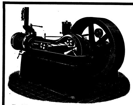
The Oiling System of our engines consists of an oil reservoir, piped to a sight feed valve at each bearing, one valve controlling the supply to all bearings. The main bearing has self-oiling rings in addition to the sight feed valve. The crank pin is oiled automatically by oil from main bearing, and also by a
