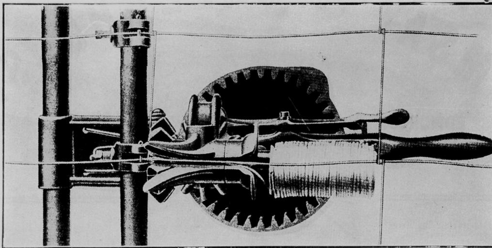
The weaving gear of the London Machine which puts the "stays" on "London" Fence "to stay."
