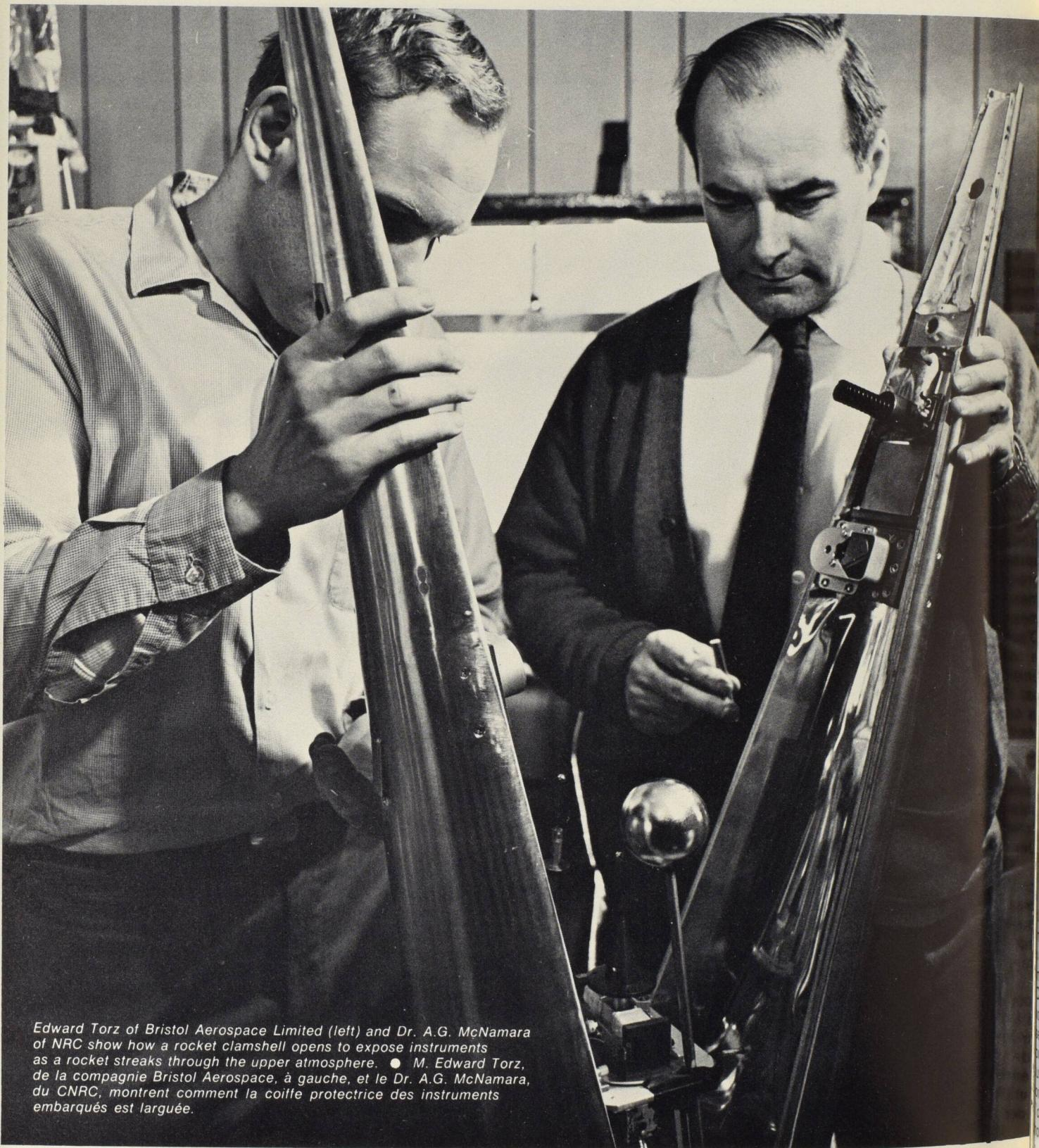
Edward Torz of Bristol Aerospace Limited (left) and Dr. A.G. McNamara of NRC show how a rocket clamshell opens to expose instruments as a rocket streaks through the upper atmosphere. ● M. Edward Torz, de la compagnie Bristol Aerospace, à gauche, et le Dr. A.G. McNamara, du CNRC, montrent comment la coiffe protectrice des instruments embarqués est larguée.
