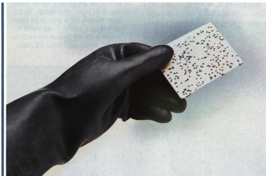
Paper chemical agent liquid detector following exposure to liquid chemical agent spray – 3-Way liquid adhesive backed.
